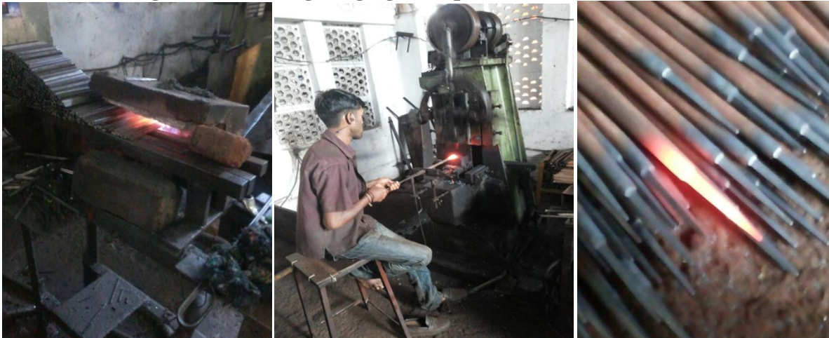
Figure No-07: Tang Forging Set Up with Gas Fired Furnace
