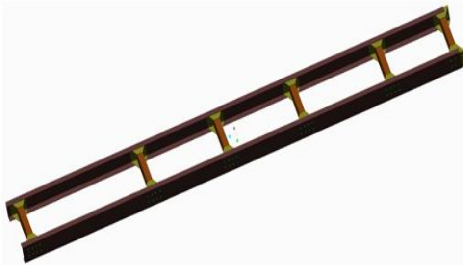
Fig. 2: CAD model of chassis in PTC Creo 3.0
